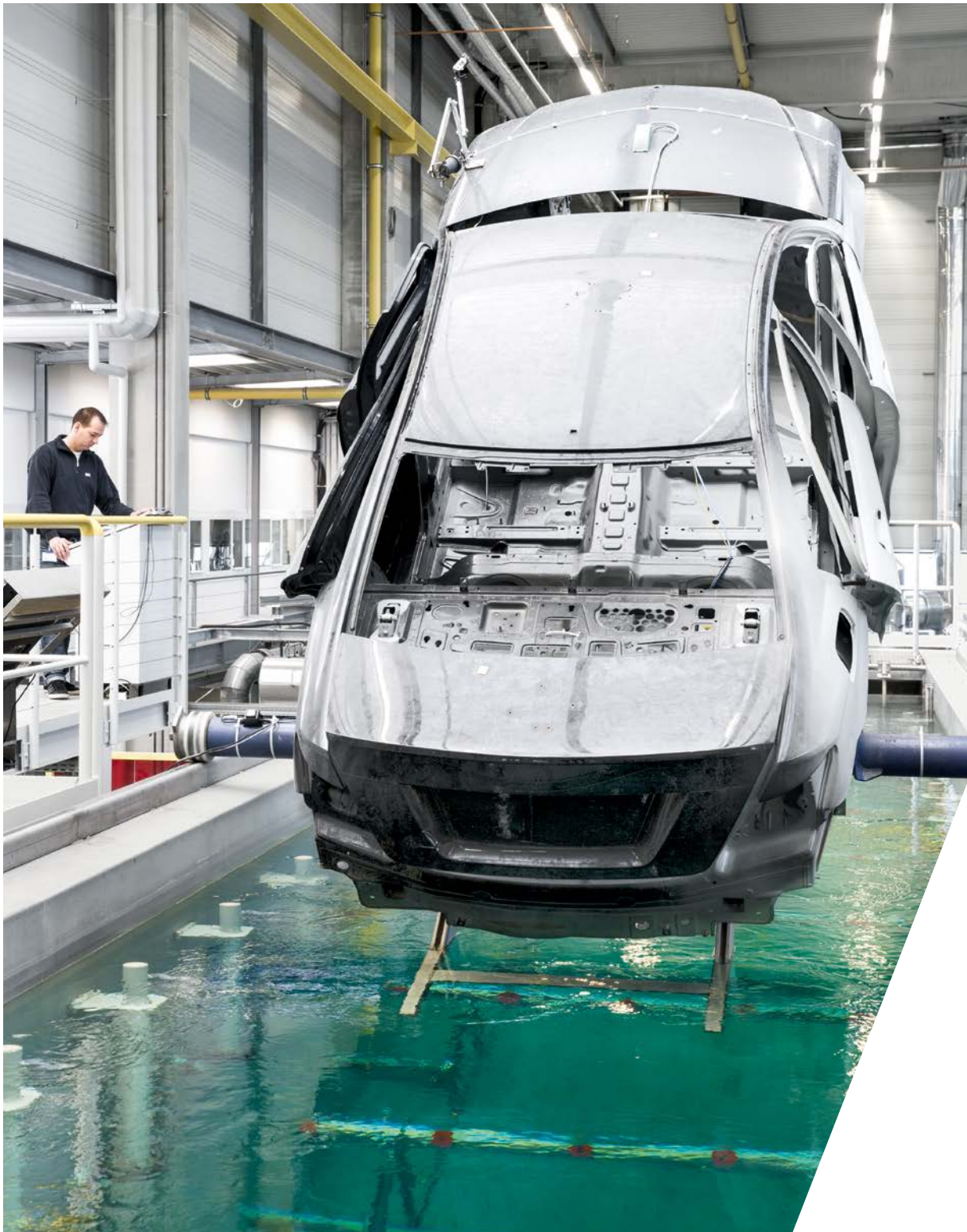
The RoDip dip-coating process is being optimized in the Bietigheim-Bissingen technology center.
