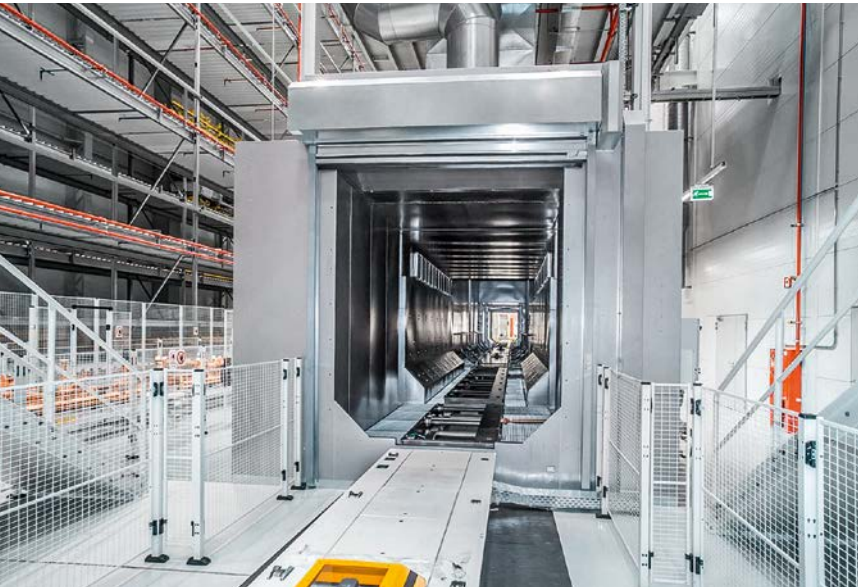
Rust doesn't stand a chance: once the anti-corrosive coating has been applied to protect its cavities, the body makes its way to the oven at 75 to 100 degrees Celsius.
