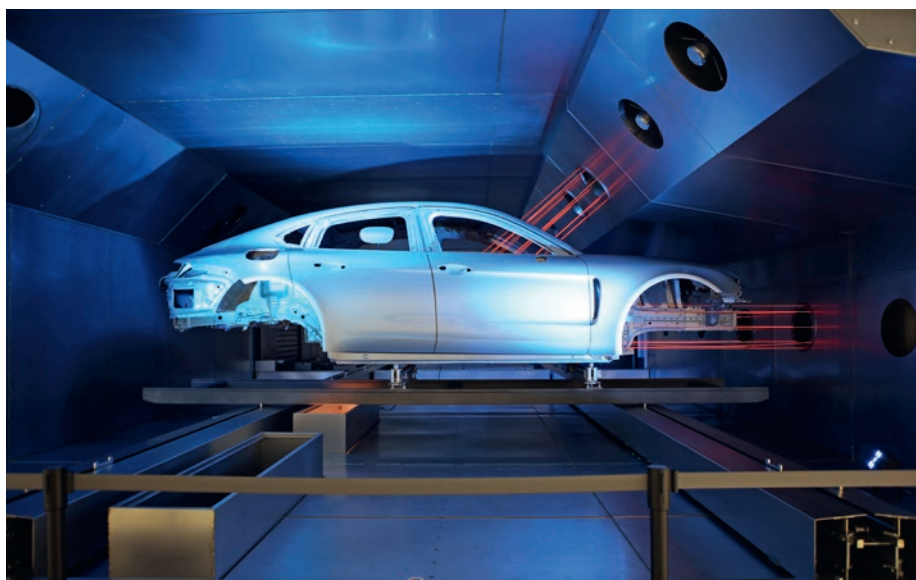
In the EcoInCure oven, the hot air flows into the interior of the car body, ensuring optimal heat transfer to parts that are difficult to access.
