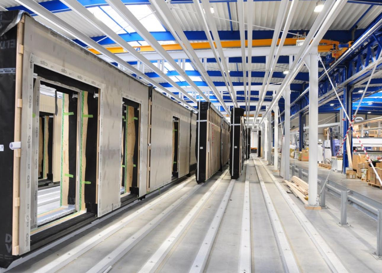
The wall modules produced by Nokera await their deployment at the construction site.
